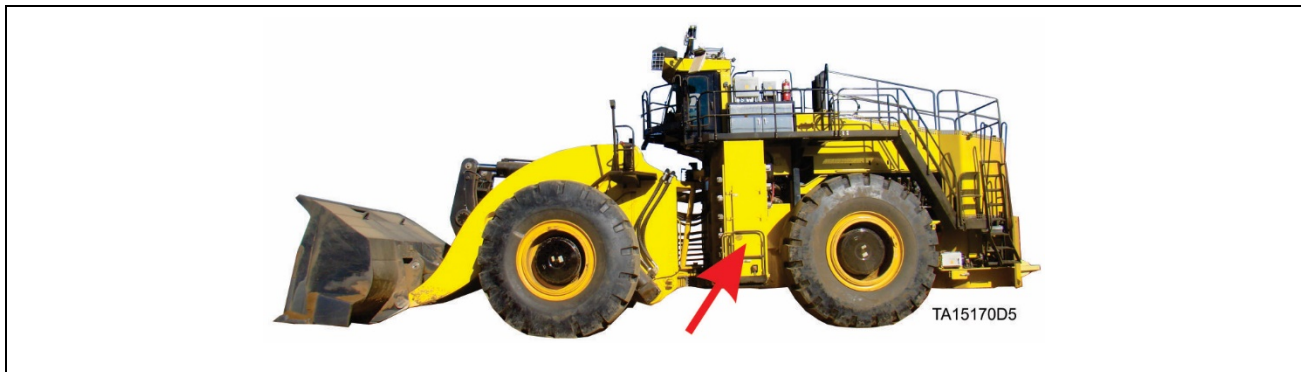
Figure 25. Electrical converter cabinet (typical)
