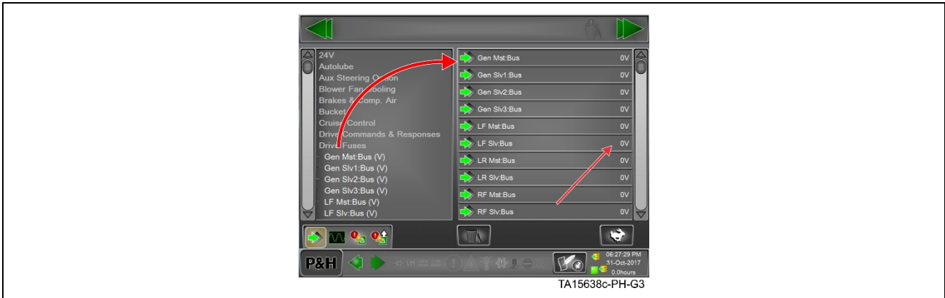
Figure 11. Bus voltage indication
