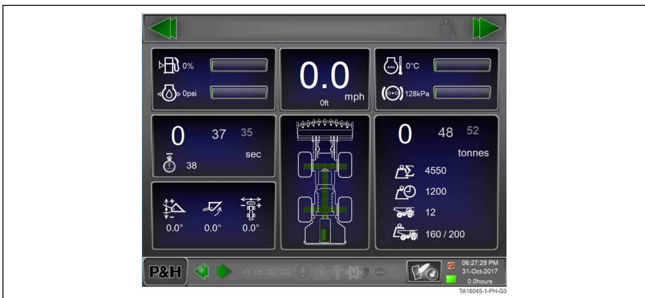
Figure 2. Operators Screen – KESS at 60%
