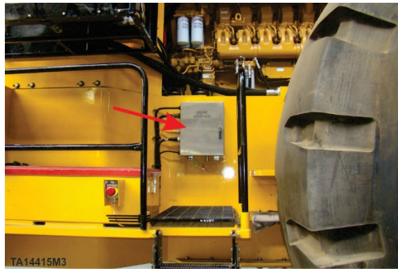
Figure 21. Typical engine interface box and typical locations
